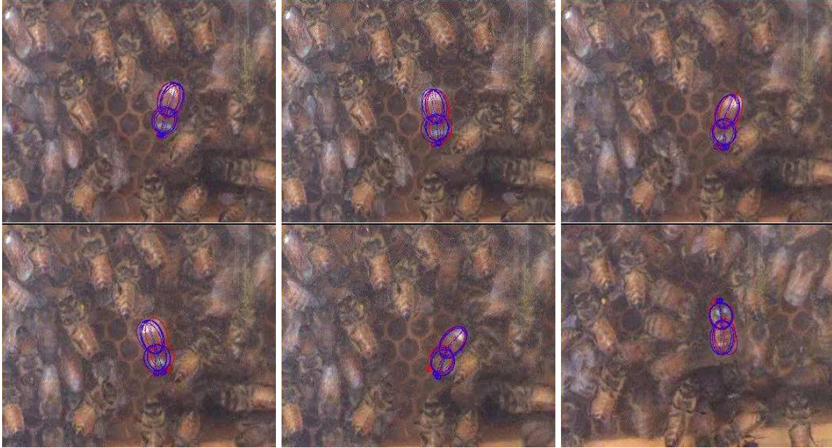
Figure 7. Sample Frames from a tracked sequence of a bee in a beehive. Images show the top 5 particles superimposed on each frame. Blue denotes the best particle while red denotes the fifth best particle. Frame Numbers row-wise from top left :30, 31, 32, 33, 34 and 90. Figure best viewed in color. (Image courtesy of Veeraraghvan et al. 15 )
